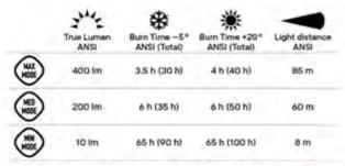
Lumen, burntime and light distance are measured according to the AND FU STANDARD
